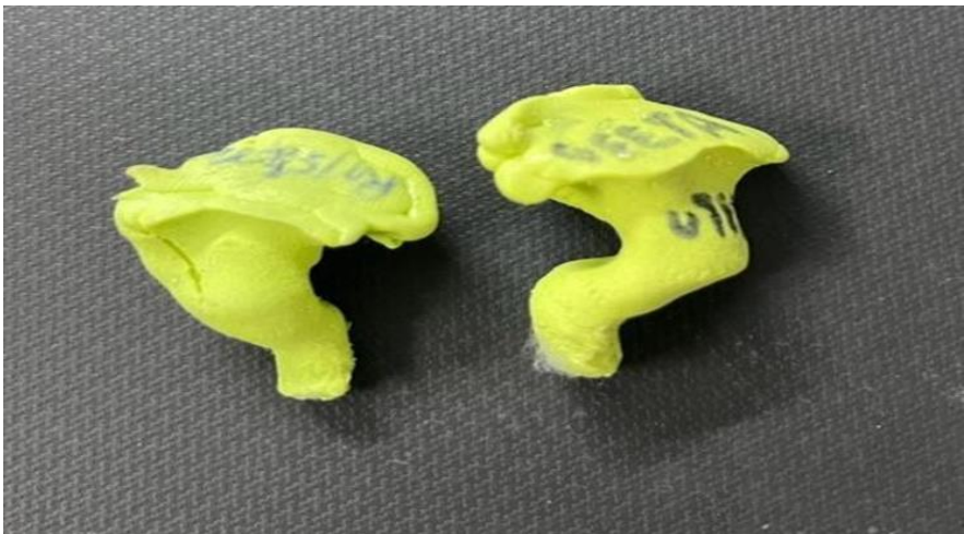
Figure 1- Silicone mold used for EAC diameter measurements.
